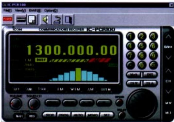
This panel contains a comprehensive set of controls such as you would find on an advanced communications receiver, including a large frequency readout, band scope, S-meter and keypad.
