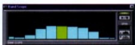
The bandscope shows signal conditions around a specified frequency.
